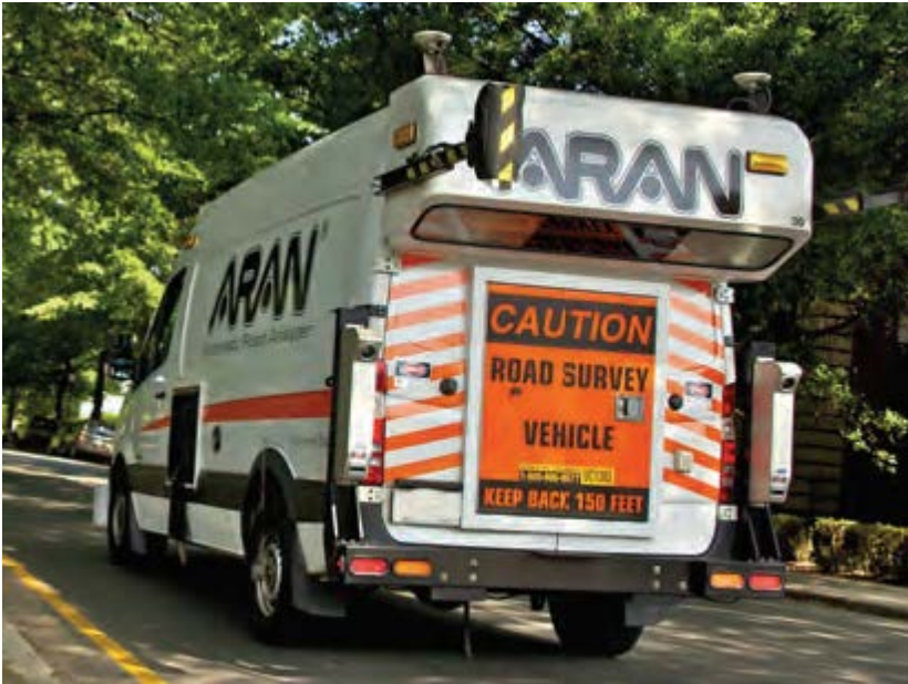
Figure 3: An Example of Roadway Data collection by Fugro Roadware-equipped Vans (Campbell, 2012)
